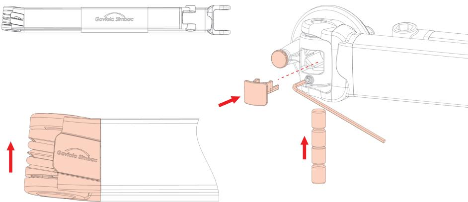
**2** Colocar la brida en la barra de carga y atornillarla a la regleta sin apretarla a fondo. Place the flange in the frontal profile and screw it to the adjustment without tightening too much.
