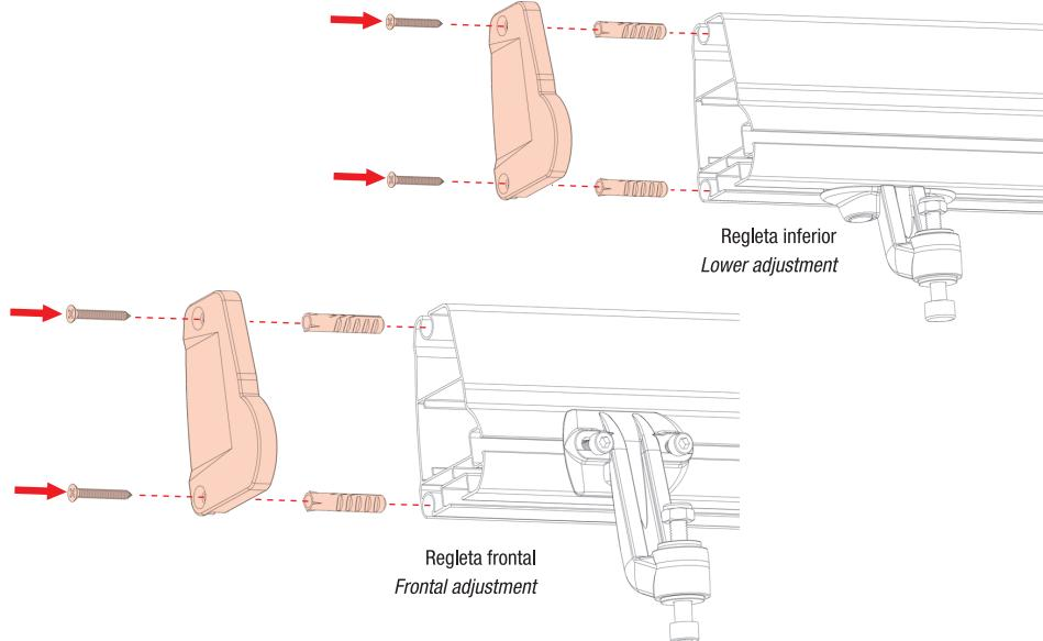
**4** Colocar la regleta en el terminal delantero y atornillar. Place the adjustment in the frontal profile and screw.
